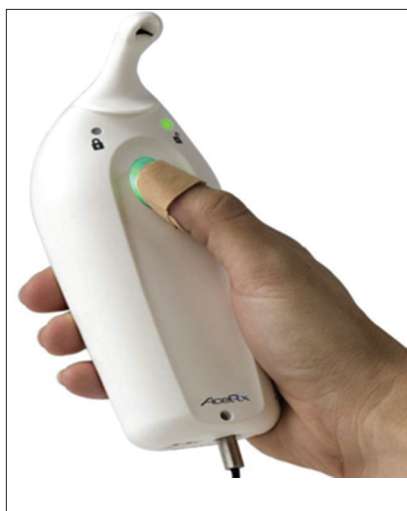
Fig. 1: Zalviso™ handheld sufentanil sublingual micro tablet system with security tether and radio-frequency identification thumb tag for single patient identification
