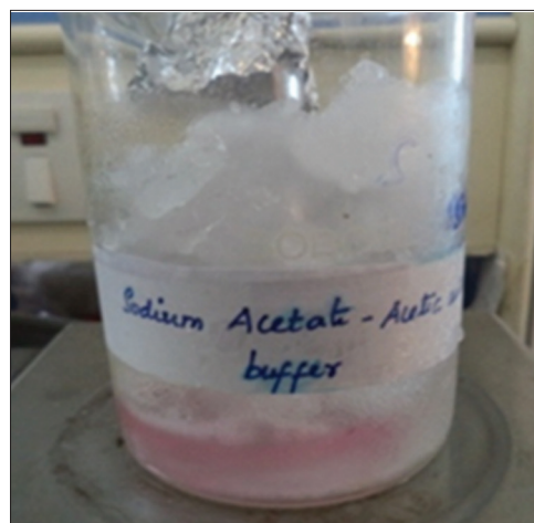
Fig. 5: Ammonium sulfate precipitation using magnetic stirrer at 250 rpm
