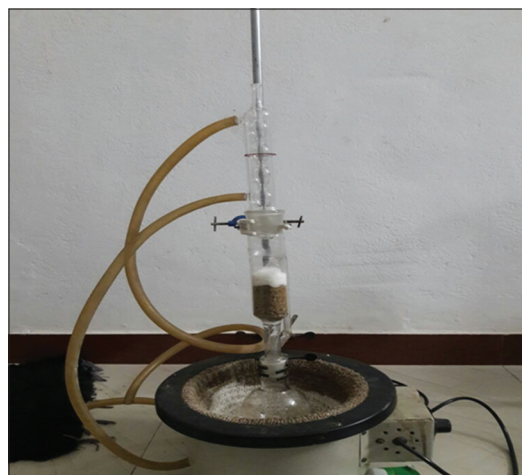
Fig. 4: Extraction of sample in soxhlet apparatus
