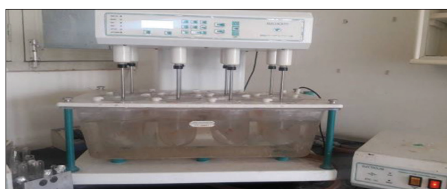
Fig. 3: Paddle over disc method for drug release studies of transdermal patches
