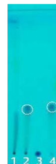
Fig. 1: Flavonoids monitoring by TLC, i.e. extract (1), ethyl acetate fraction (2), distilled water fraction (3), and quercetin (4)
