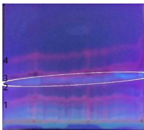
Fig. 3: Preparative TLC chromatogram showed 4 bands with ethyl acetate: n -hexane (8:2) as mobile phase
