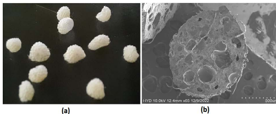
Fig. 1: Images of Topotecan loaded chitosan based floating microspheres. (a) Photographic image; (b) SEM image of the cross-sectioned microspheres indicating inner pores as cavities (at 65x magnification)
