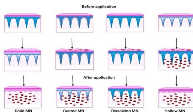
Fig. 3: Different types of microneedle drug delivery approaches [22-25]
