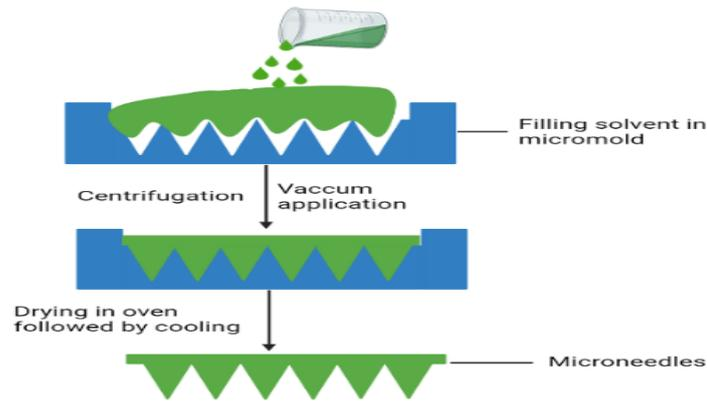
Fig. 4: Micromolding method [26]
