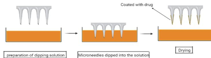
Fig. 6: Dip coating method [28]
