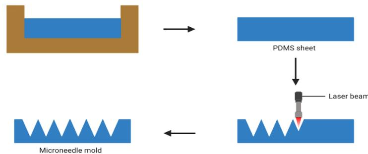
Fig. 5: Laser cutting method [27]
