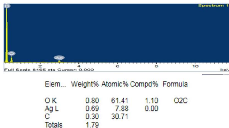
Fig. 2: EDX of synthesized silver nanoparticles from Premna integrifolia
