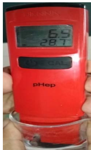
Fig. 5: pH meter measuring surface pH of the film
