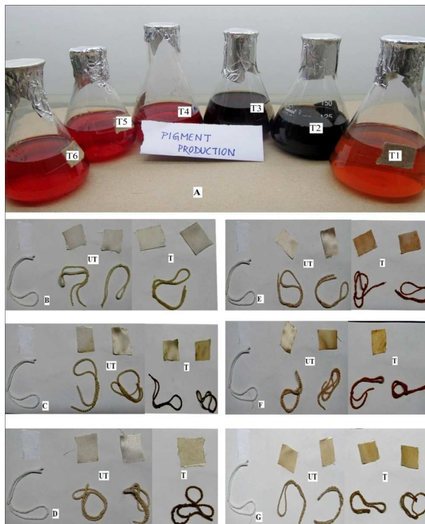
Fig. 7: A. Pigments after removal of fungal biomass (T1-T6); B-G: Dyed samples (T1-T6) with control, T: treated with mordant; UT: untreated
