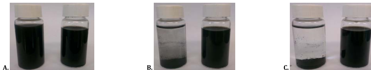
Fig. 7: Photographs of pristine-CNT (left) and CNT-COOH (right) suspensions in deionized water. After A) two hours B) 24 h and C) two months of resting
